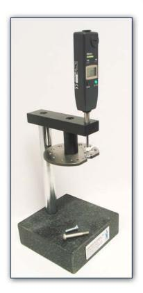
This gage is designed to measure the protrusion height of flat head screws and the head heights of non-flat head screws with accuracy and speed. The protrusion heights are measured by placing a flat head screw in the appropriate gaging hole and positioning it under the indicator foot for measurement after having "Zeroed" the indicator on the gaging plate surface. The foot is raised. The screw is placed in the "V". The foot is rested on the screw's head and the measurement is taken.
