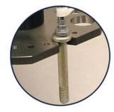
When ordering Protrusion-Head Height Gages, specify dial indicator (.001 "resolution) or electronic indicator (either .0005" or .0001" resolution) and the gaging plate you require. Gaging plates can be quickly changed on the same gage.
